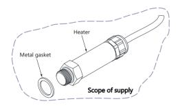
Connect to the inlet at the bottom of the housing using a metal gasket. If the inlet is on the underside of the housing, connect it using an additional "tee" to the inlet.
